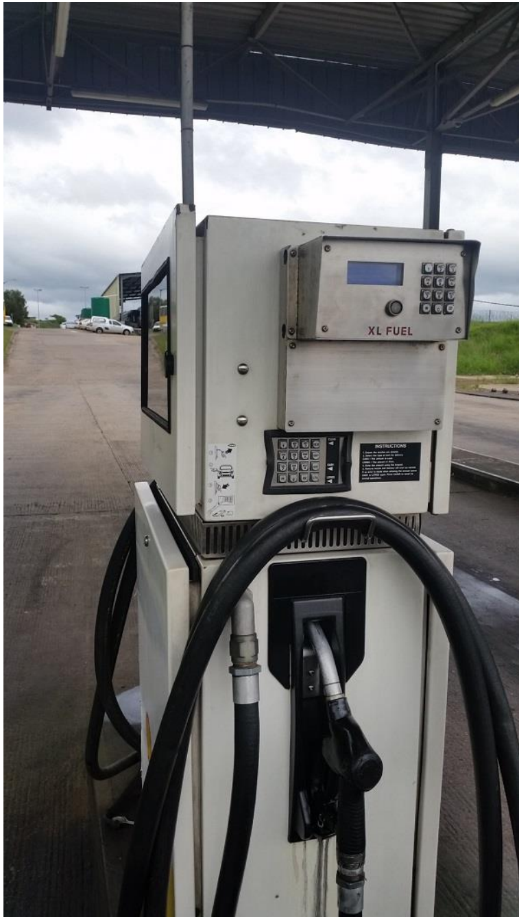
Figure 1 XL Fuel control unit mounted on a fuel dispenser
